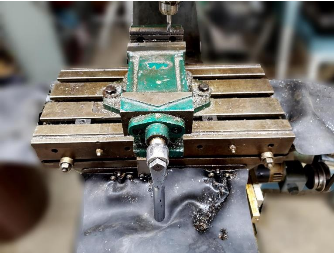
Figure 2: Becker mill with imported 4" vice and original handle
