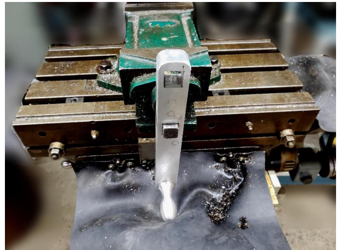
Figure 3: Becker mill with finished speed handle
