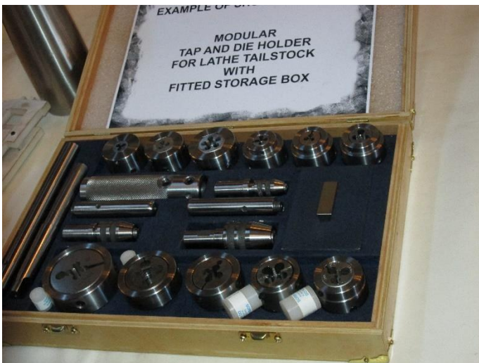
Lathe tailstock tap and die holders built by Vernon Eshbaugh, one of our NEMES members.
