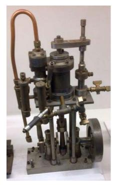
I think this is a lubrication pump. There is no power takeoff pulley, the crankshaft does nothing but spin the flywheel. The shaft coming out the top of the steam cylinder has a link to the shaft to the right. That shaft is a plunger into the small cylinder below that must contain a small piston for pumping oil or water. There must also be a check valve on the pump input side so that liquid is sucked into the cylinder from the input side and then pushed out the output side.
