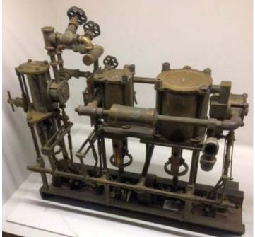
Like the engine at the right end of the display, this is also a compound steam engine, intended to power a boat. It could be a model, but it looks kind of industrial, so I think it might be a real full size engine for propelling a small boat.
