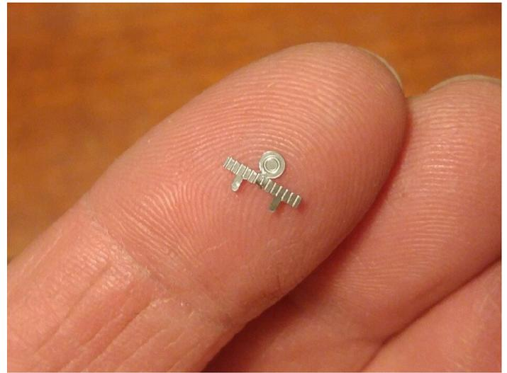
I use the cutters to remove the etches from the sheet, hold them in the pliers so the edge of the part is parallel to the edge of the pliers, and use the needle file to file off the sharp barb left from removing the piece from the sheet. If you look at the above photo, you can see where I had to file just below the circular part, about 1/2 way between the two tabs.
