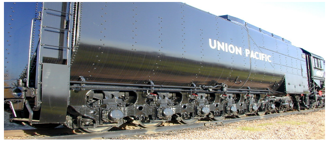
This image of engine 4023's tender helps illustrate why the type is known as a centipede tender. Visible on this side are the five wheels mounted to the tender and the two installed in the leading truck. The diagonal row of rivets indicates the partition between the water tank in the rear of the tender and the coal bunker in the front. Note the recessed ladder on the left and the 10 in (254 mm) sideboards atop the tender on the right. ( Larry Pieniazek image via Wikimedia Commons )
