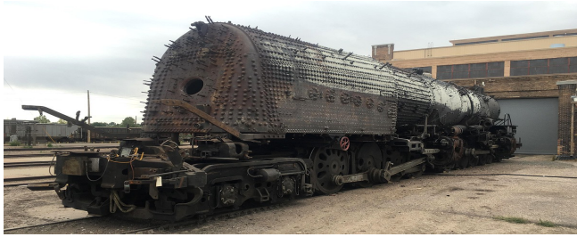
Big Boy 4014 sits in Cheyenne undergoing restoration. The cab has been removed, and the locomotive has been stripped down to the boiler. (Union Pacific image)
