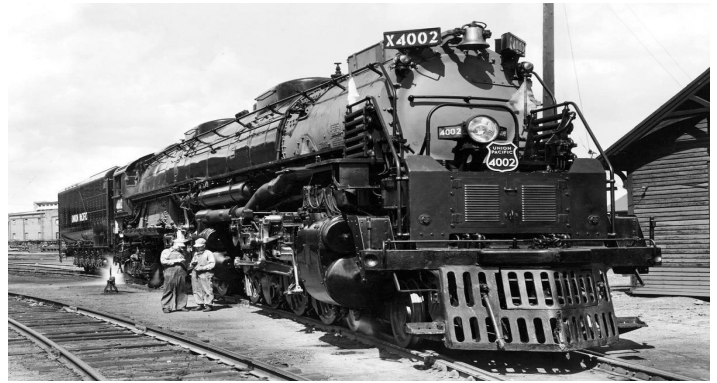
The crew standing next to newly-completed Big Boy 4002 gives scale to every part of the engine: the cylinders, wheels, boiler, etc. The railing on the front of the -1 class engines was originally coolers for the air pump. The -2 class used a standard Wilson aftercooler, as the custom set up on the Class -1 would often crack. As the coolers failed on the -1 class, they were removed and replaced by Wilson units. (Union Pacific image)
