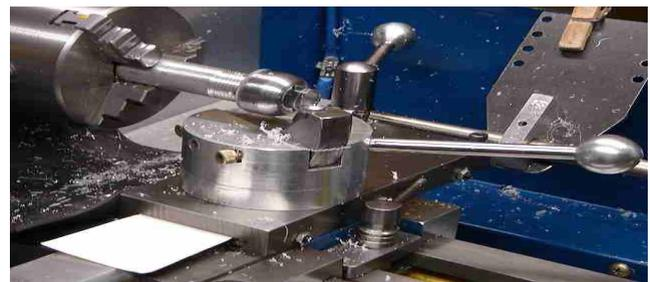
Face the flat end (bottom) of the optic first, polish it as described above, then turn the 3/8" section of the optic to fit the base using low RPM and lubricant. Most any tool can be used to rough the 3/8 section but the cutoff tool works well to finish it because it has little rake; take
