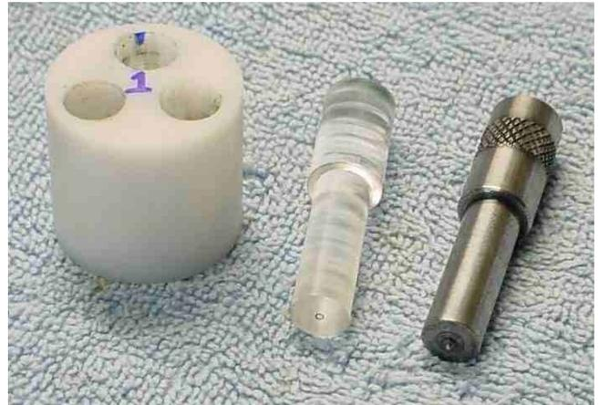
An optical punch is helpful in placing a punch mark accurately on a scribed point. A center punch can then be used to enlarge the mark. My unit is based on one shown on Harlan's Site(Disappeared 3/13).
