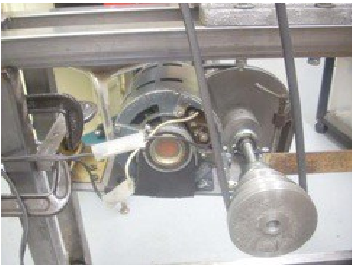
Motor & Jack Shaft Photo by R. G. Sparber
