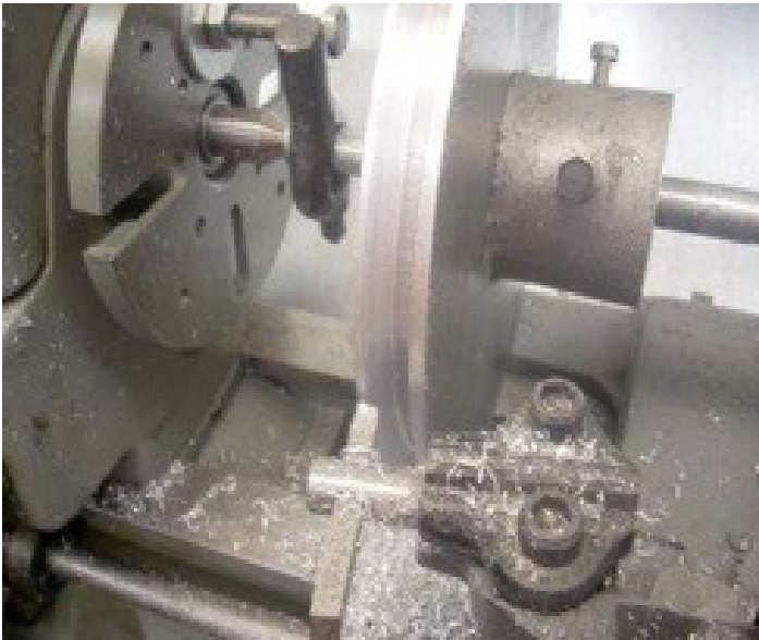
Cutting V Groove Photo by R. G. Sparber
