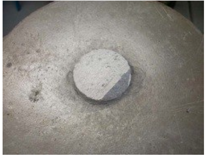
Sprue Removed Photo by R. G. Sparber
