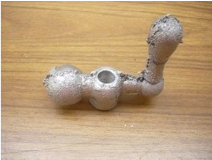
Casting Drilled Photo by R. G. Sparber
