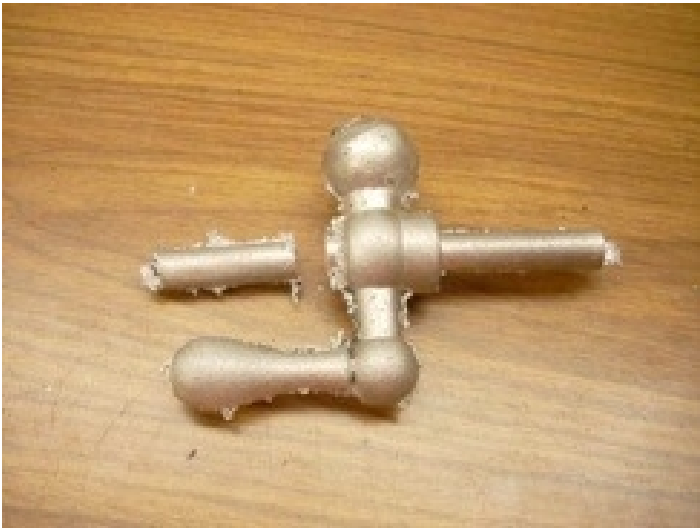
Casting After Rod Cut Photo by R. G. Sparber
