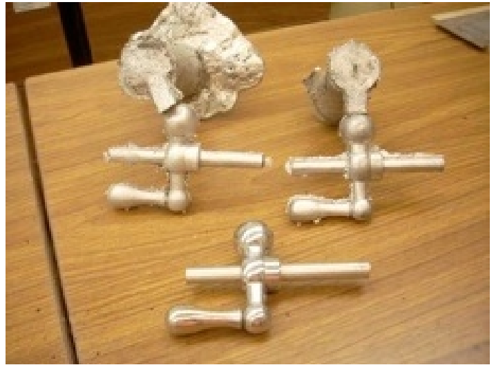
Pattern & Two Castings Photo by R. G. Sparber
