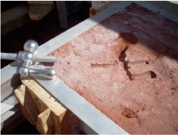
Cavity in Drag Photo by R. G. Sparber
