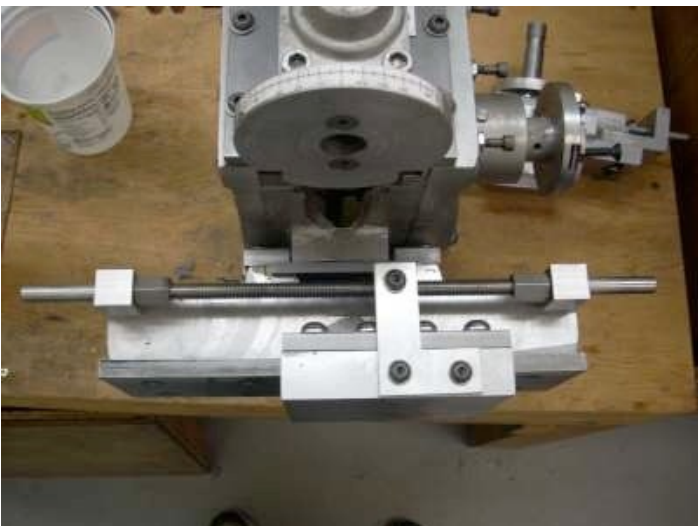
Cross Slide Top View Photo by R. G. Sparber
