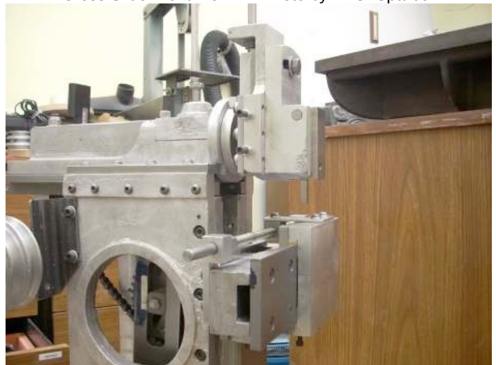
Cross Feed Side View Photo by R. G. Sparber
