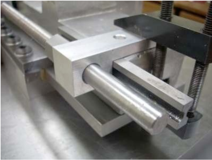
Right Bearing Block Photo by R. G. Sparber
