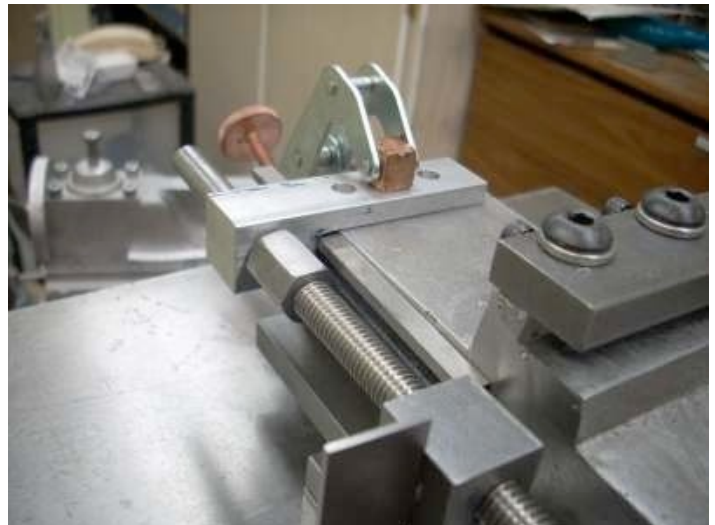
Left Bearing Block Photo by R. G. Sparber
