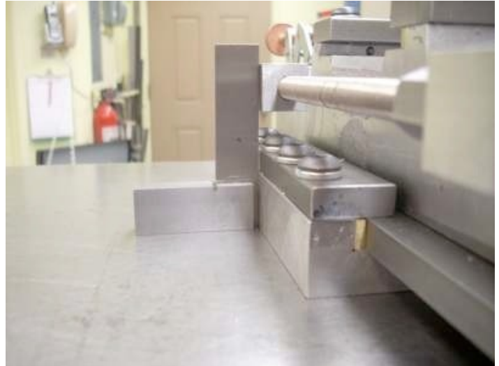
Positioning Bearing Block Photo by R. G. Sparber
