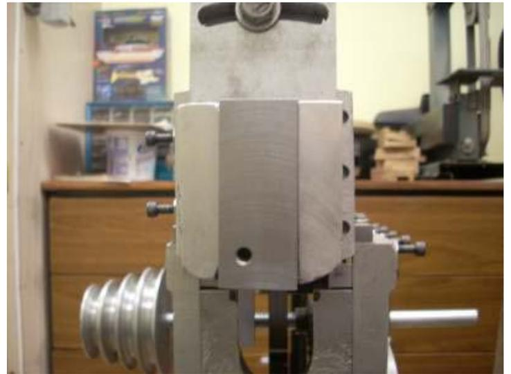
Clapper Set Screw Hole Photo by R. G. Sparber
