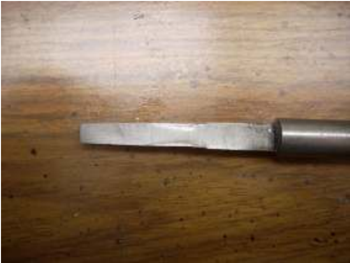
Reamer Damage Photo by R. G. Sparber
