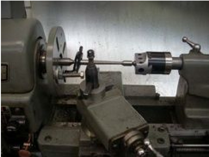
Cutting Taper Photo by R. G. Sparber
