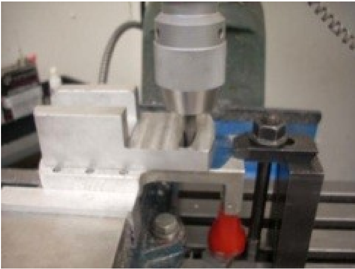
Drill Clamp Bolt Hole Photo by R. G. Sparber
