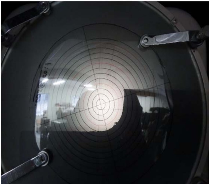
Profile of half the addendum curve with radius chart.
