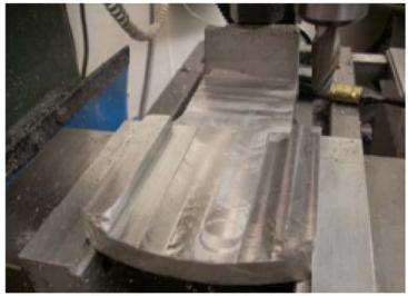
After Milling Photo by R. G. Sparber The end mill was then set to be 0.02" below the wear pads and the remainder of the surface cut.
