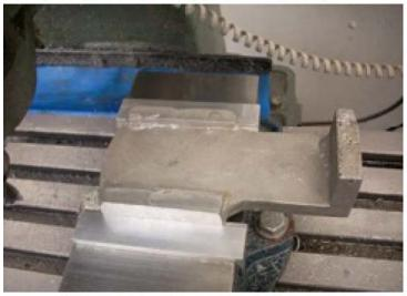
Mill Setup 4 (Almost) Photo by R. G. Sparber The casting is now securely held by my soft jaws on Reference 2 and 2 prime. Reference 1 is parallel to the mill table.
