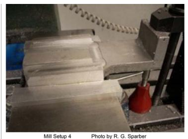
A jack is snugly placed under the end of the casting and a hold down clamp added. You can barely see the slide pads that have just been cut with an end mill. This is zero reference for my Z axis. I then raised the cutter 0.240" and cut the clamp support blocks. That leaves 0.010" for shims so I can accurately adjust the distance from the underside of the clamps and the top side of the slider.
