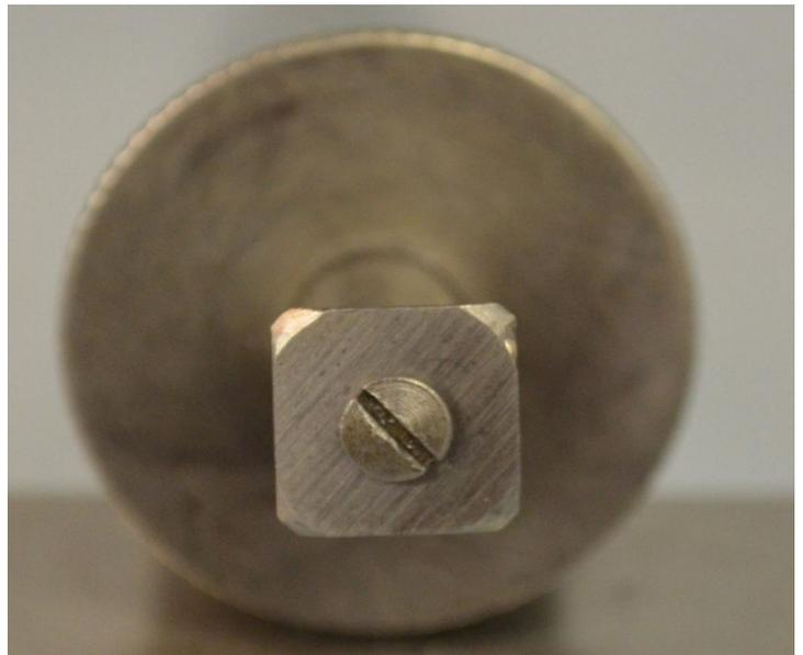
Make the cutter from a piece of 1/32" thick O1 tool steel. The edge length of the square cutter should be about 1/8" more than your beam diameter. Drill and countersink the cutter for a small flat-head screw. Harden the cutter and then temper it for one hour at 375° F to get a hardness of around 60 Rockwell C.
