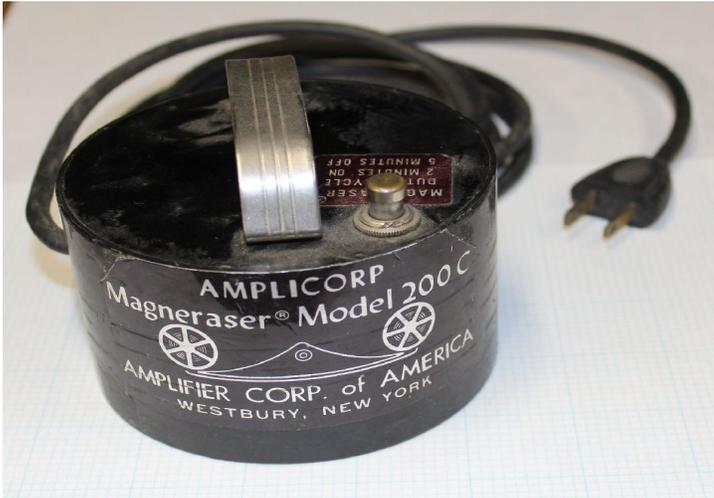
This larger demagnetizer is made for 10½” reels of tape and is equally powerful and useful, just a bit larger, so takes up a little more room on the shelf:
