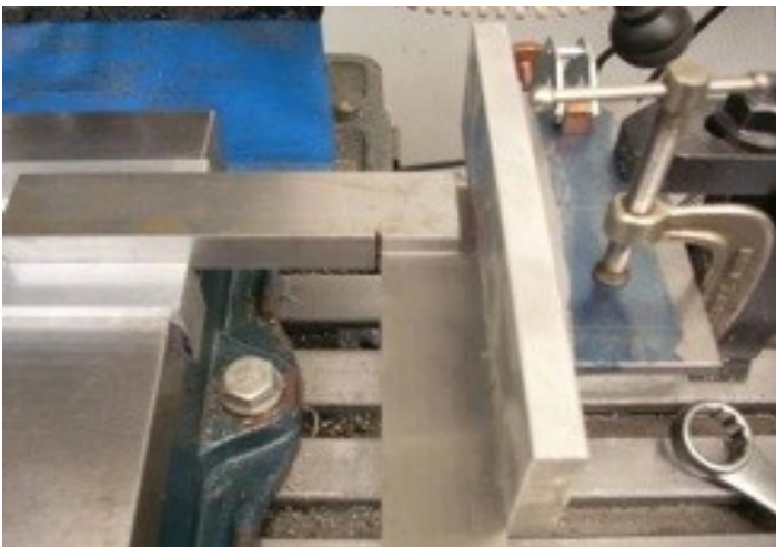
Aligning on Mill - Photo by R. G. Sparber
