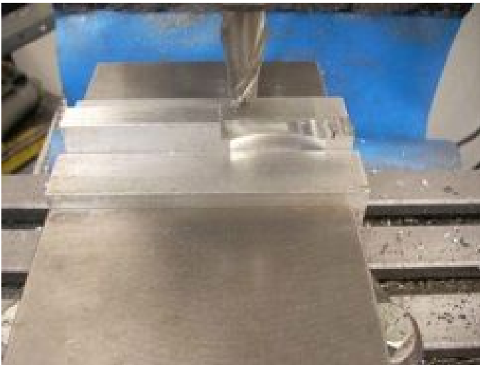
Milling Width Photo by R. G. Sparber
