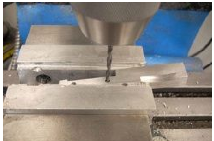
Clearance Drilling Photo by R. G. Sparber
