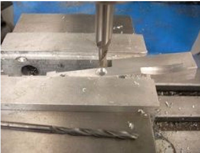
Drilling with End Mill Photo by R. G. Sparber
