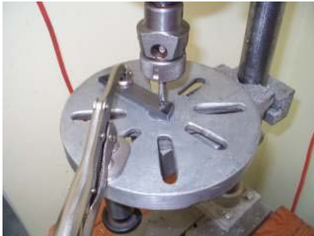
First Clamp Method Photo by R. G. Sparber
