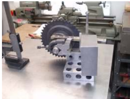
Laying Out Sprocket Photo by R. G. Sparber
