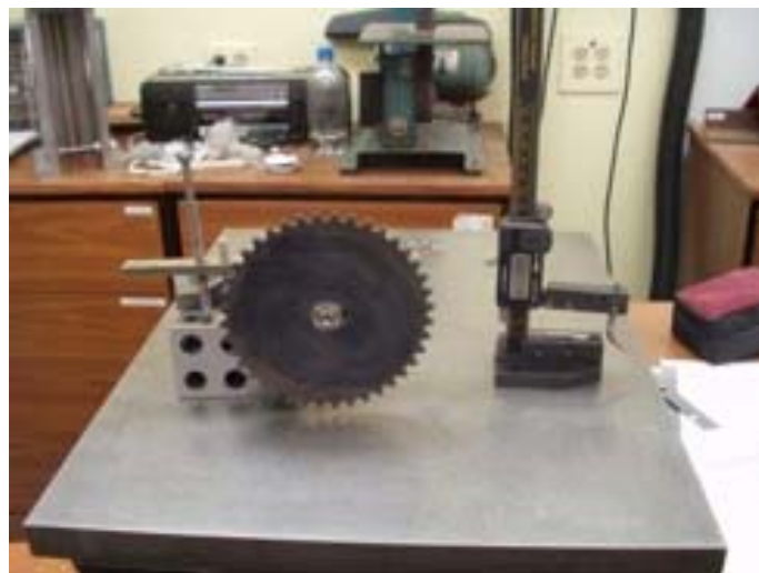
Scribing Sprocket Photo by R. G. Sparber
