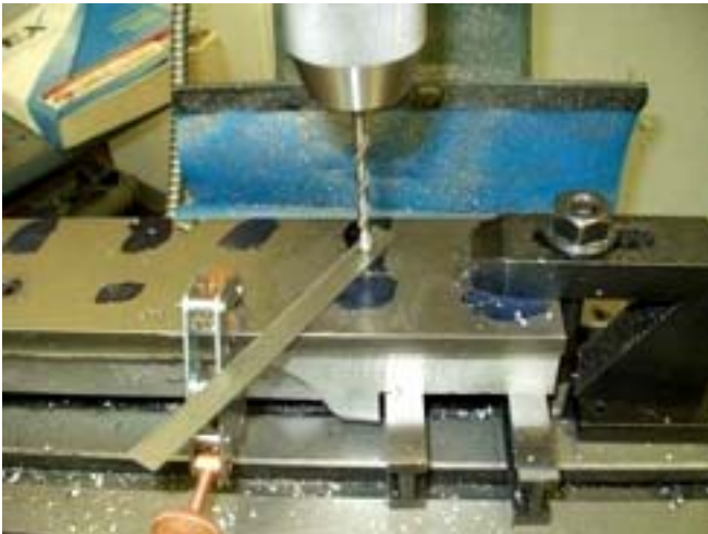
Zeroing Z Axis Photo by R. G. Sparber
