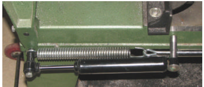
Bandsaw modified with a pneumatic damping cylinder
