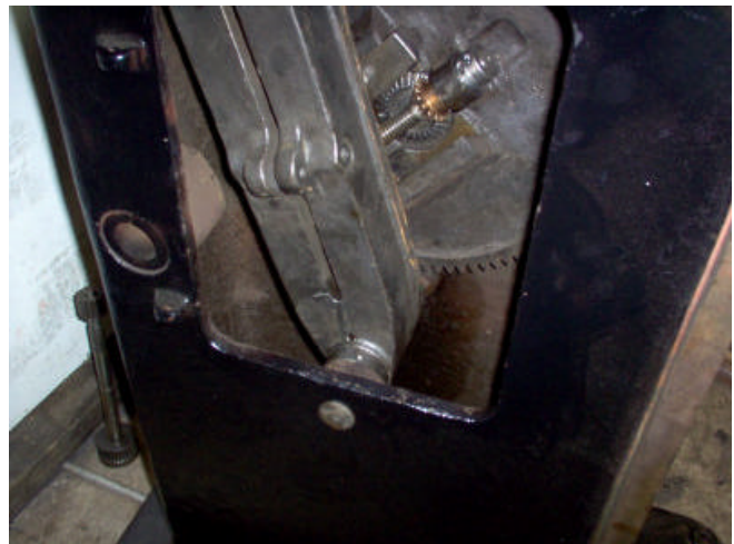
Install Rocker Arm Photo by Eric Lavelle
