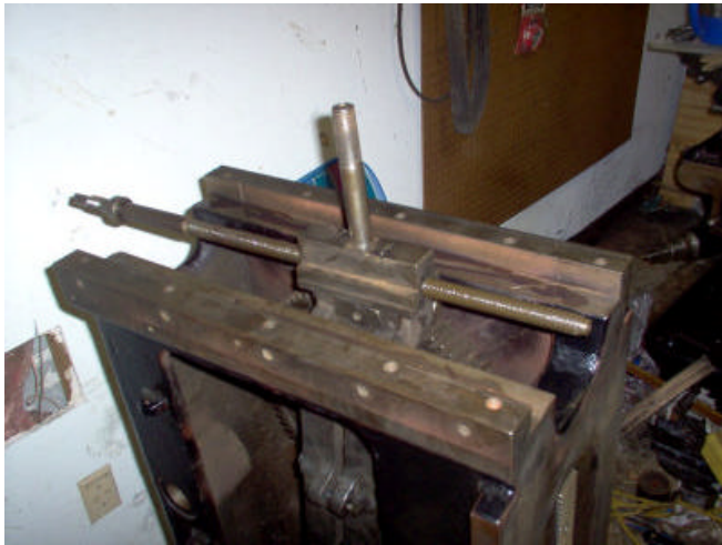
Install Ram Lead Screw Photo by Eric Lavelle
