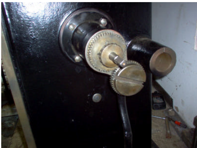
Install Auto Feed Gears Photo by Eric Lavelle
