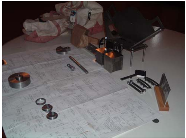
Errol Groff is working on this Ray Hasbrouck designed Steam Engine. It requires no castings and is designed to be used in a boat.
