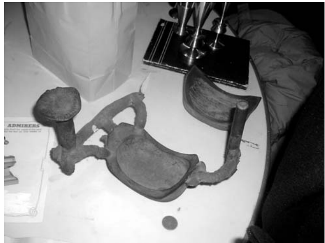
A bronze casting of a sand dome for a 1" scale Pacific Locomotive made by visitor and Waushakum Live Steamer Joe Ng.
