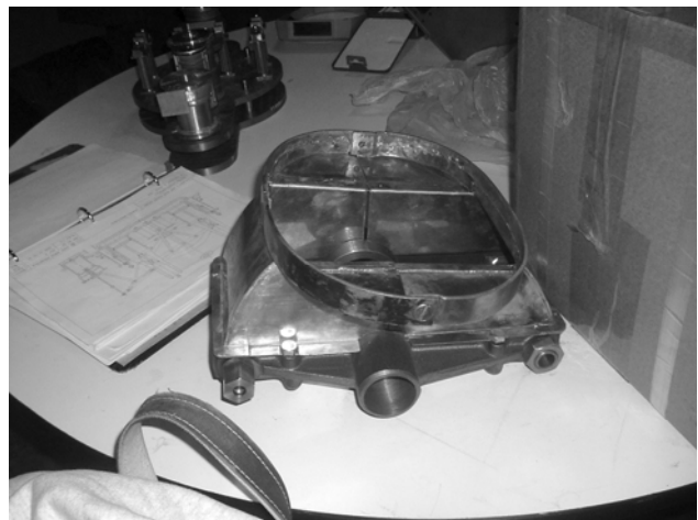
A formed copper shroud, built by Rollie Evans, made for enclosing the crankshaft of a Stanley steamer engine.
