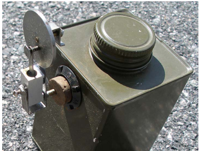
"Can" engine, oscillating steam. Boiler was made from a metal screw-top can he used for solvents.
