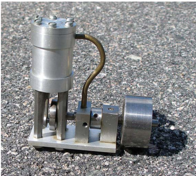
Hit-or-miss, hopper cooled farm engine, the Associated Mfg. Co. "Hired Man". The castings are from Paul Breisch & Sons Model Works. Flywheels are 6" in diameter.
