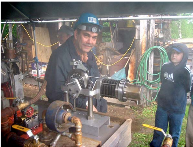
Ed Seldin with his new stirling cycle engine
