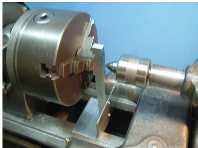
Norm's Tool Height Fixture - Calibration to perfect height with a live center
