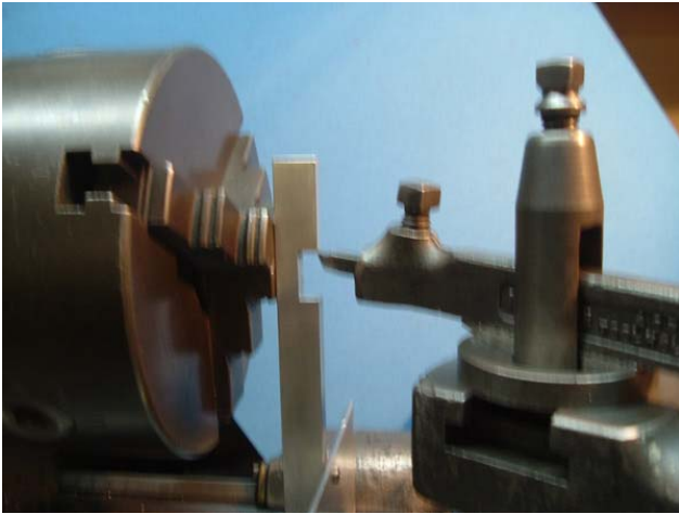
Norm's Tool Height Fixture – In use
