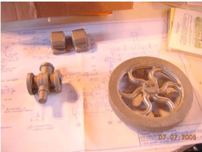
Patterns for an oscillating steam engine:
