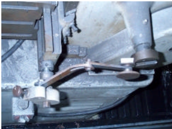
Damaged feed link
