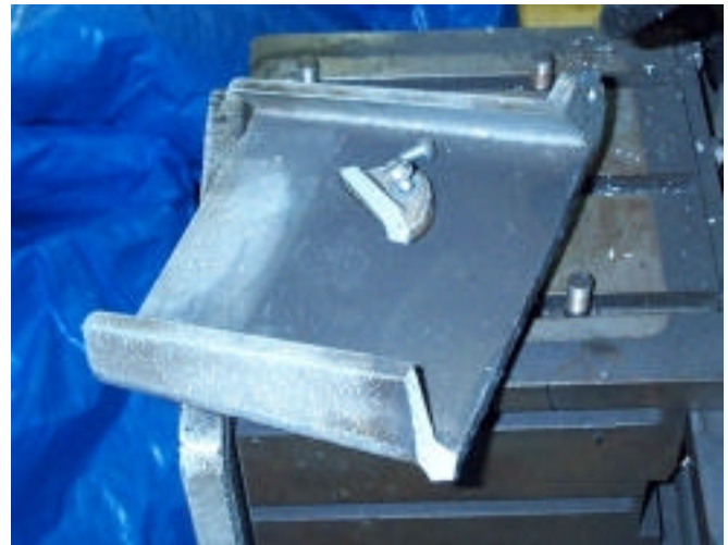
Damaged ram guard
