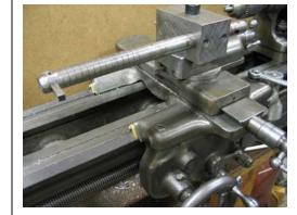
Fig. 5 Boring Bar Overhang
