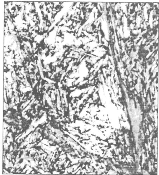
Figure 15-3.—Microscopic structure called martensite magnified 2,500 times.
