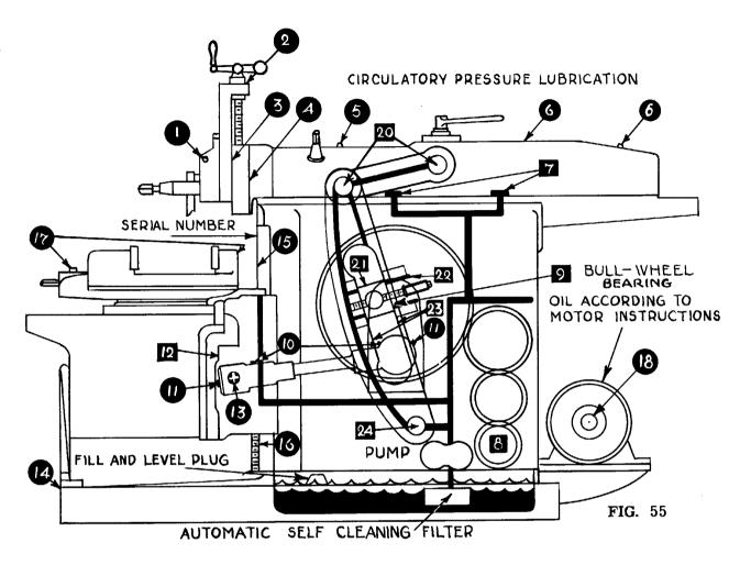
NOTE: All places on a shaper which must be lubricated in one way or another have been located and numbered on the oiling chart shown above. In addition, corresponding numbers precede the directions for oiling these places. The numbers for those places which are usually oiled automatically are enclosed in a square instead of a circle.
