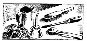
another must be lubricated also. When starting work on a shaper, the operator should locate all the bearing surfaces. If the bearings are hand oiled, he must determine the location of the oil holes for these bearings and make certain that they are kept well oiled at all times. If they are automatically oiled, continuous circulation of oil must be maintained. The entire circulatory oil
