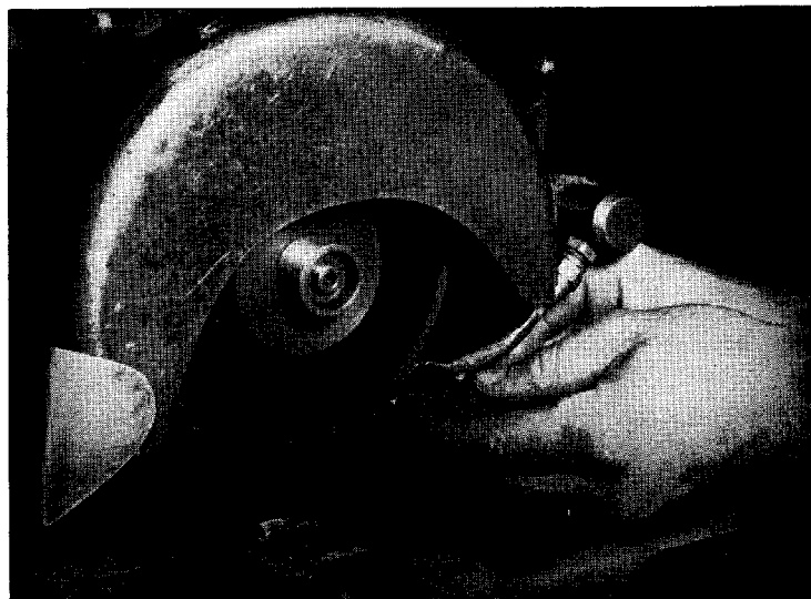
Opening up the cutting face of a vitrified bonded diamond wheel with a Crystolon stick after truing
