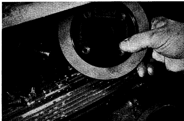
A popular shape and size of metal bonded diamond wheel for sharpening carbide single-point tools
