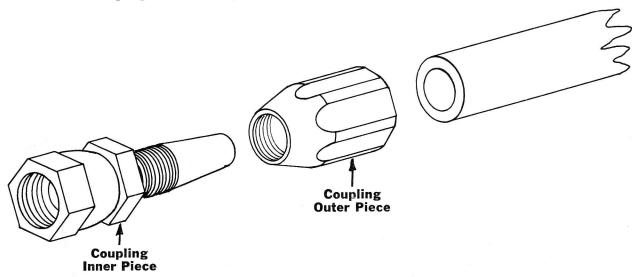
2.27 Reassembling is done in the following manner. First screw the outer piece on the hose, in a counterclockwise direction, until it seats firmly against the hose. Back the coupling off  $\frac{1}{4}$  turn. Place a small amount of grease 90 weight, on the tapered inner piece and screw the two pieces together. The outer and inner piece properly installed will seat together. Blow out the inside of the hose so no dirt will be introduced into the system.
