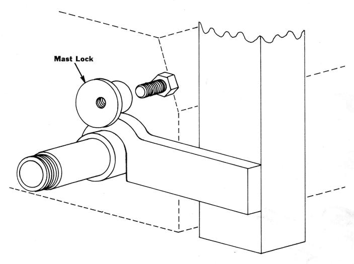
1.11 The mast lock bolt is located inside the drive motor compartment just above each drive motor mount. Loosen each bolt. Make sure the mast is seating properly on axle housing and tighten the bolt letting the mast mounting plate hold the eccentric lock from turning. This method of tightening insures the mast lock from loosening due to pressure from the mast.
