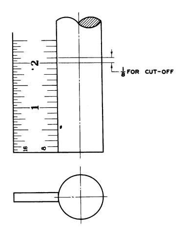
1. How much stock is required for 4 pieces of C. R. S. 2½" long, if 1/8" must be allowed for each piece for cutting off?
