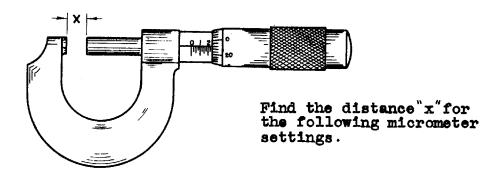
NOTE: Where possible, secure a micrometer, set at the indicated positions, and note the reading in each instance.
