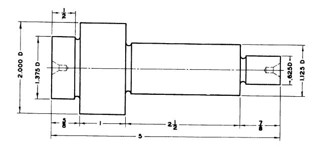
The above spindle must be rough turned, annealed, finish turned, hardened and tempered, and ground.
