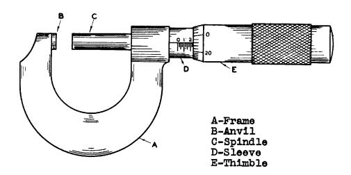
The spindle C is attached to the thimble E on the inside. The part of the spindle which is concealed within the sleeve and thimble is threaded to fit a nut in the frame A. The frame being held stationary, the thimble E is revolved by the thumb and finger, and the spindle C being attached to the thimble, revolves with it and moves thru the nut in the frame, approaching or receding from the anvil B.
