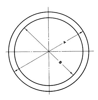
On the piece to be turned, if the existing diameter A is measured and the finished diameter B is known, what is the depth of the cut?
