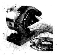
The interchangeable mask plates, which can be switched in seconds, remove all possibility of error, insuring accurate spacing and rapid indexing.
