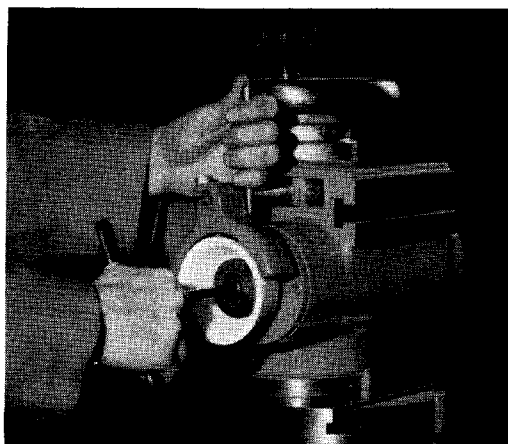
Figure 24B Grinding Wheel Collets are Quickly Interchanged by Removing Socket Head Screw
