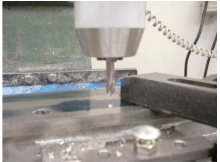
Center Drill 2nd Hold Photo by R. G. Sparber
