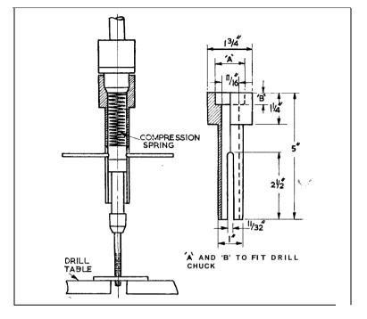
dimensions *A* and *B*. This should be a firm non-sloppy fit over the nose of the chuck.
