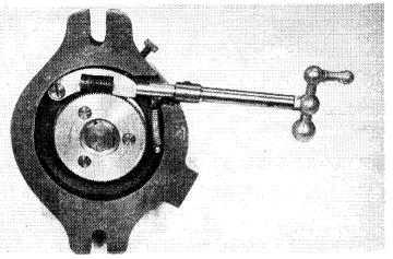
Underside of the rotary table, with the spring-loaded quick-release worm gear
