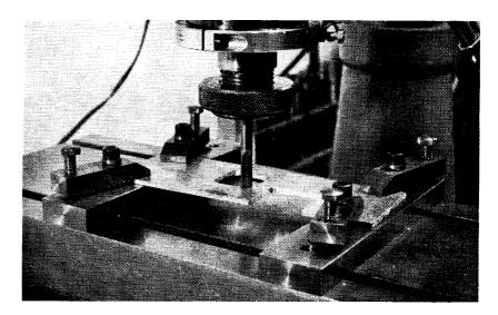
Using the clamping fixture to hold work for the cutting of holes in sheet metal
