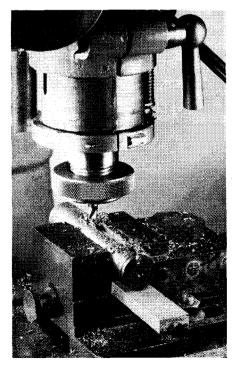
Milling a keyway fin. wide X tin. deep with a slot drill in a single cut
