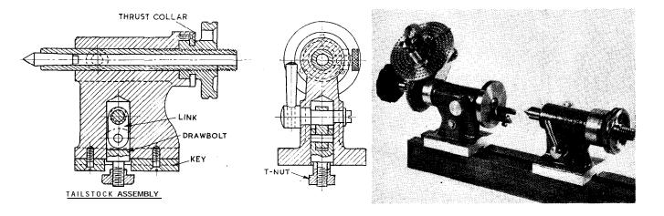
be used for finishing if it does not have to take out more than a few thou. At the same setting the back edge of the base, the shouldered end of the headstock, and the recess in the tailstock boss, can be machined. Mandrels, of the two appropriate sizes, may be used to mount the castings for facing off the front ends, and the front edge of the base, which should be flush.
