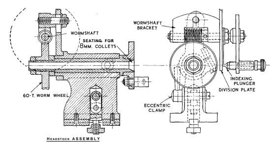
similar, they will be dealt with as a pair. The first task in each case was the boring of the main housing. It was carried out by mounting the casting rear end outwards in the fourjaw chuck, with one of the jaws reversed. If the chuck is not large enough to hold the work comfortably, an alternative method would be to clamp it by its flat base to an angle plate on the faceplate.
