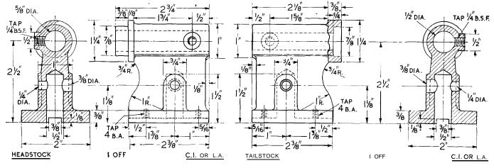
must be drilled vertically in the casting to take the drawbolt. This can be done in the vertical milling machine, while the two components are set up on the jig; or alternatively, they may be set up singly on an angle plate in the lathe.
