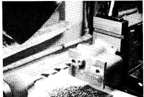
Fig. 9: Drilling bolt holes.
