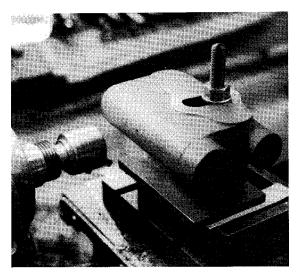
Fig. 7: Flycutting setting edge of block.
