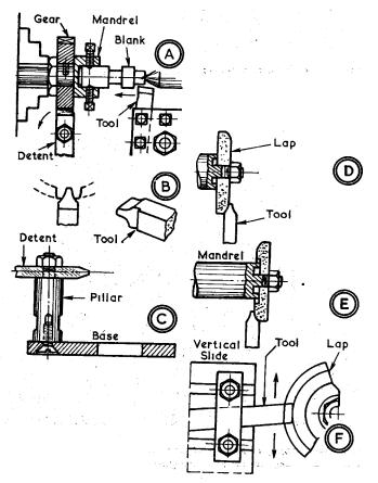
pattern to make a form tool to plane a pinion with 12 teeth, or vice **versa**, for the two tooth shapes are entirely different.
