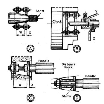
with the bore of one of the washers, the bulb lights up. By noting the light, or lack of it, as the tool is moved in the washers, you know how to set the slide. To make a check of concentric spinning, turn the chuck with the tool inside one of the washers.
