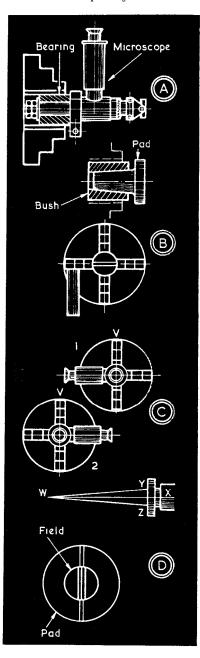
illustrated at diagram B. The pad is turned from mild steel with a taper for the tailstock barrel. Then it is mounted in a bush in the four-jaw chuck. This bush should be bored in the chuck to take the pad. The scribing tool is set just above (or below) centre height, and a stop is used to two opposite jaws of the chuck. By this method, the lines must lie equally each side of the axis.
