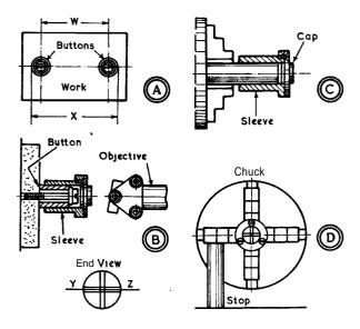
spin truly to a test indicator. The work may be clamped to the faceplate or on an angle plate; or it can be held in the independent chuck.
