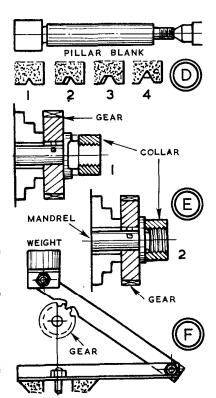
leaves them with half-circles YZ. Finally, each piece is held in the chuck to skim its inside face for clearance.
