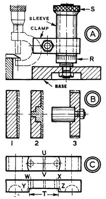
measure them in the normal way. When you need 2 in. with the spindle right up, you use a 1 in. block with a flat pointer on top to set the anvil, as shown. If you want 3 in., you build up 2 in. with a pair of 1 in. blocks.
