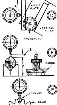
and for tapping the face of work, use a lead or hide hammer. If a faceolate wobbles. pack at the low point with paper. To true a button C, tap the edge of work with a brass or aluminium punch-the clamps can set a vertical slide to any angle just gripping. Then tighten them firmly.
