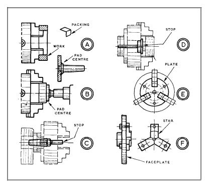
other face-the one to the steps of the jaws. In that event, a tool point or indicator may be run between the jaws for testing facial truth, although a better way is to test the faces of jaws before the work is mounted, and then pack them as necessary. This can be done with shimstock to one or two jaws, each piece being bent to a right-angle and fixed to its jaw with a strip of adhesive tape over the top.
